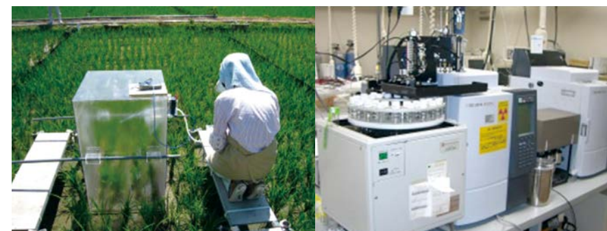
A sealed box is placed over the rice plants on the paddy surface, and air is collected from within at regular intervals (left). A sensor measures the density of three greenhouse gases simultaneously (right) to calculate emissions versus area. Source: NARO
