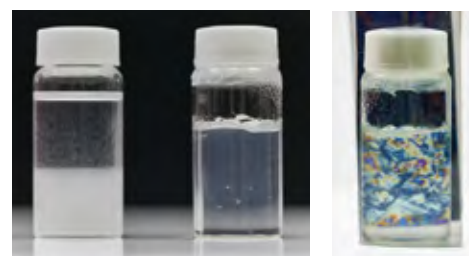
Water and ordinary pulp (left): Water and CNF mixture looks transparent (middle), but with an orthogonal polarizer, you can observe CNF dispersing (right).
