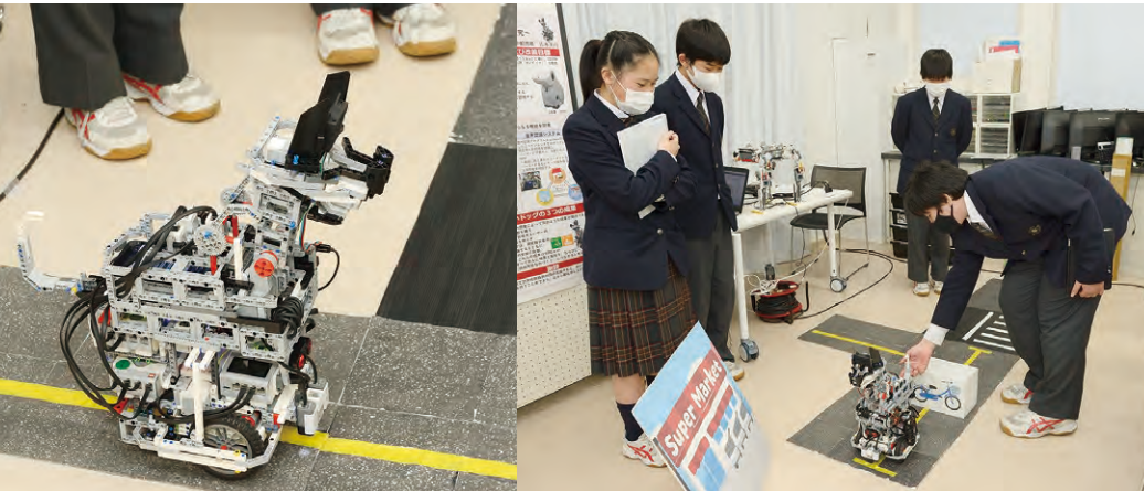
Guide Dog Robot “Ai-Dog” that automatically runs to a voice-directed destination.
